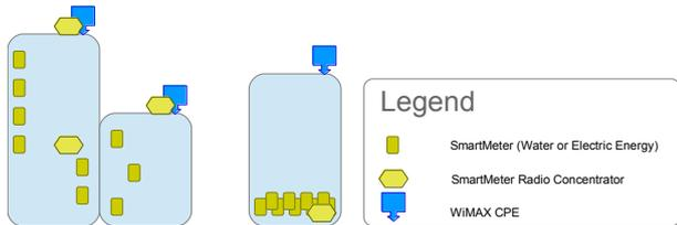
This scenario is dominated by household users, with a high density of meters. The meters can be all concentrated in cabinets in the basement or at street level; alternatively, each apartment can have its own.
